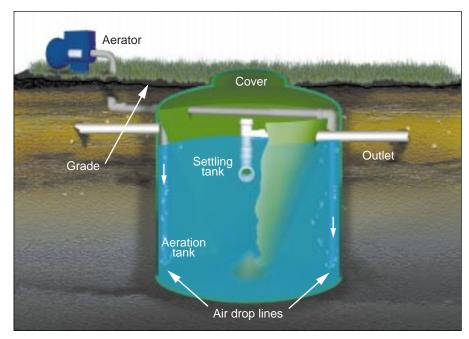
Figure 2: An aerobic treatment unit.
